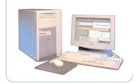
The AD952-II family of stream analyzers provides in-depth deferred analysis and comprehensive checking of MPEG-2, DVB, ATSC and ISDB transport streams. The analyzers fully support Tektronix scripting system, which enables the user to specify additional analysis functionality for use with proprietary systems.
